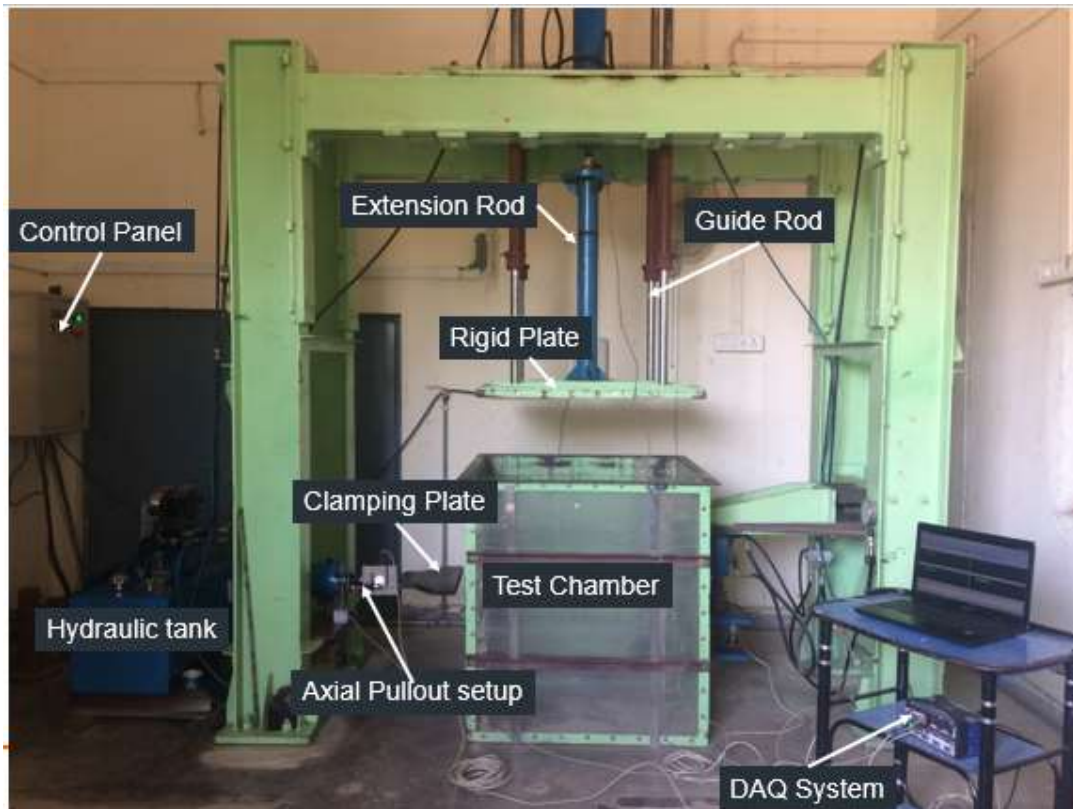
Figure 2.7 Photograph showing axial pullout test setup
