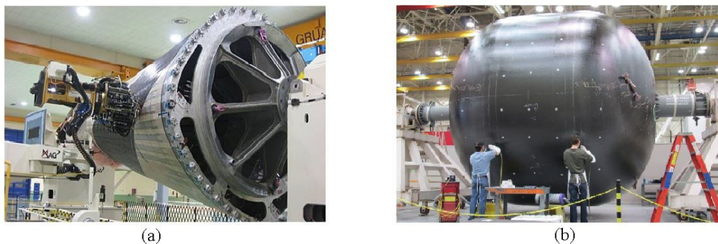
Figure 1.1: a) Composite used in fuselage of aircraft b) Composite fuel tank constructed by NASA and Boeing
