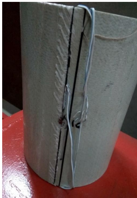
Figure 127 Failure mode in specimen 1(back side)
