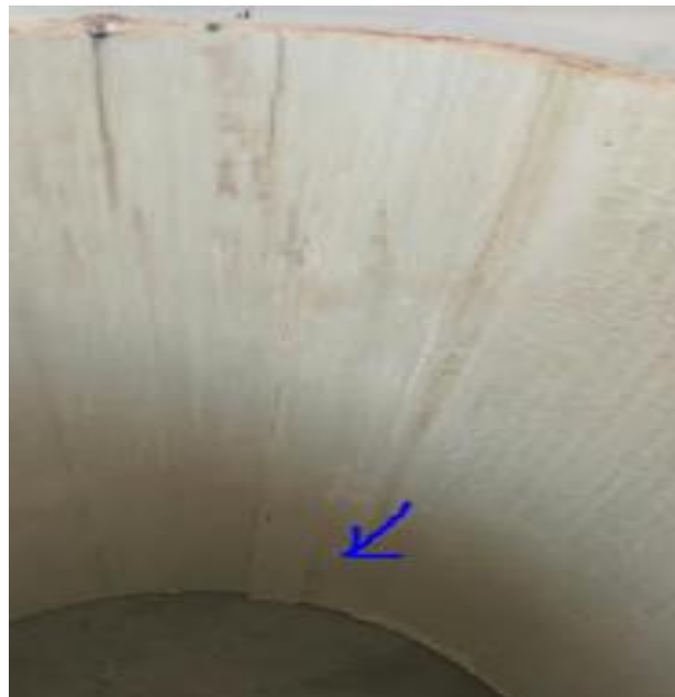
Figure 132 Delamination occurring in Specimen2
