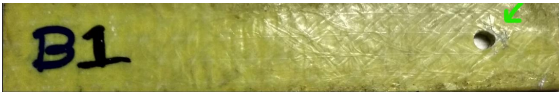
Figure 121 Bearing failure observed in b1
