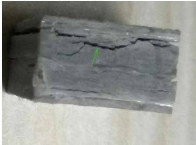
Figure 108 Rupture occurring in compression strength test for channel section specimens
