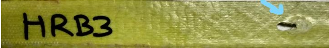
Figure 117 Shear out failure observed in HRB3
