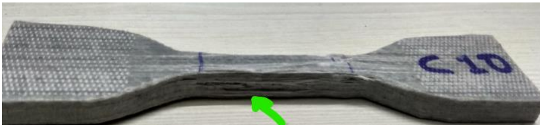
Figure 100 Delamination in channel section specimens (type four)
