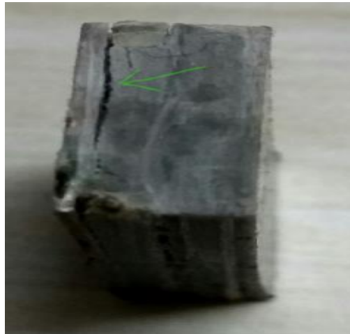
Figure 111 Rupture observed during compression modulus test of channel section specimens
