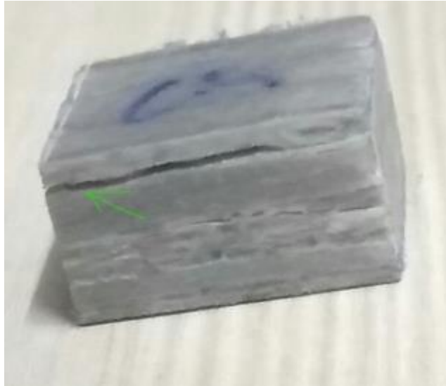
Figure 107 Delamination in compression strength test for channel section specimens
