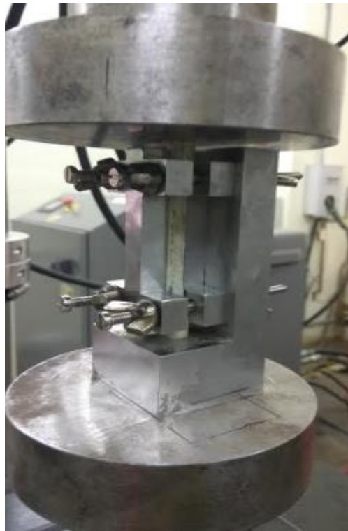
Figure 29 Fixture for compression test of coupons with jig
