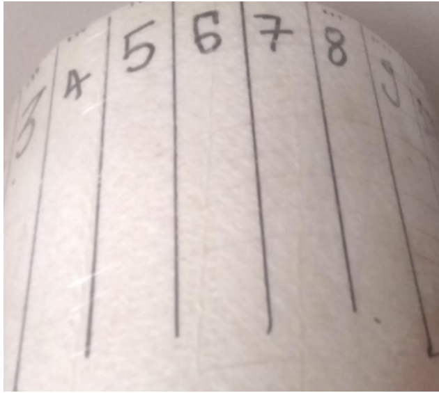
Figure 7 Pipe used for cutting coupon specimens
