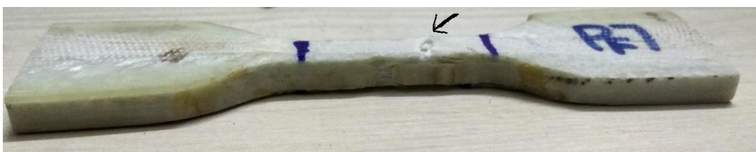
Figure 104 Shear plane rupture for pipe section specimens (type four)
