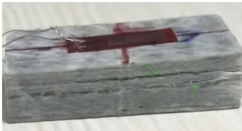
Figure 110 Delamination observed during compression modulus test of channel section specimens
