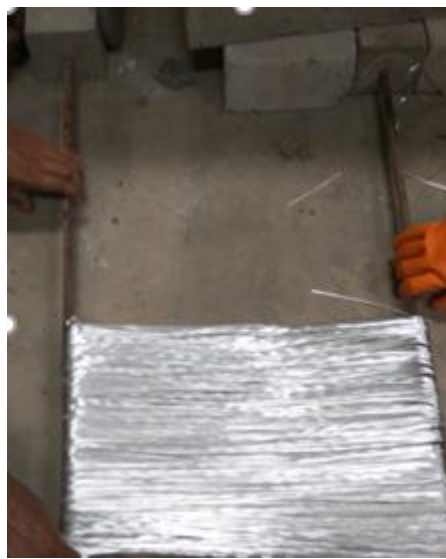
Figure 36 Tensioning of rovings done with help of steel rods
