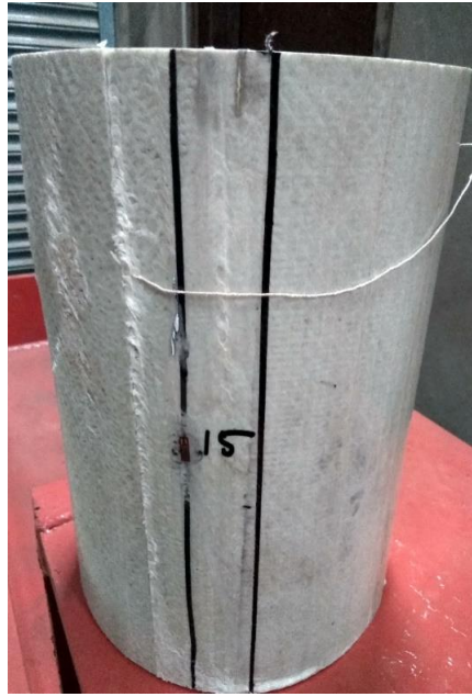
Figure 126 Failure mode in specimen 1(front side)
