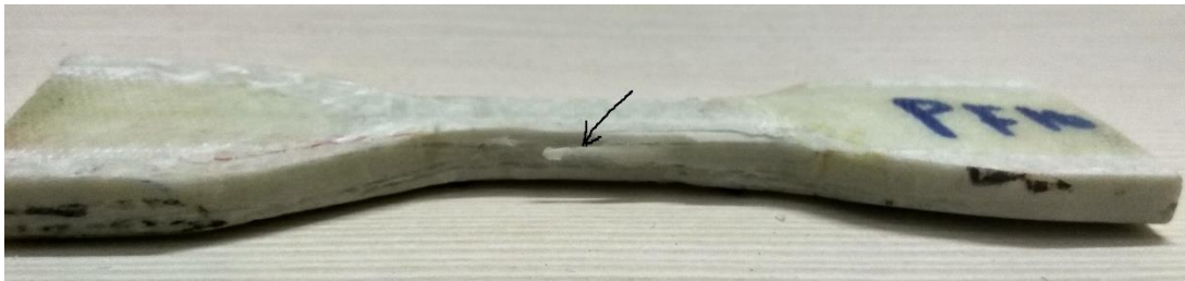
Figure 105 Delamination in pipe section specimens (type four)
