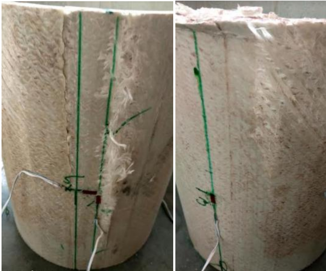
Figure 137 Failure through strain gauge 4 (left) and through strain gauge 3 (Right)
