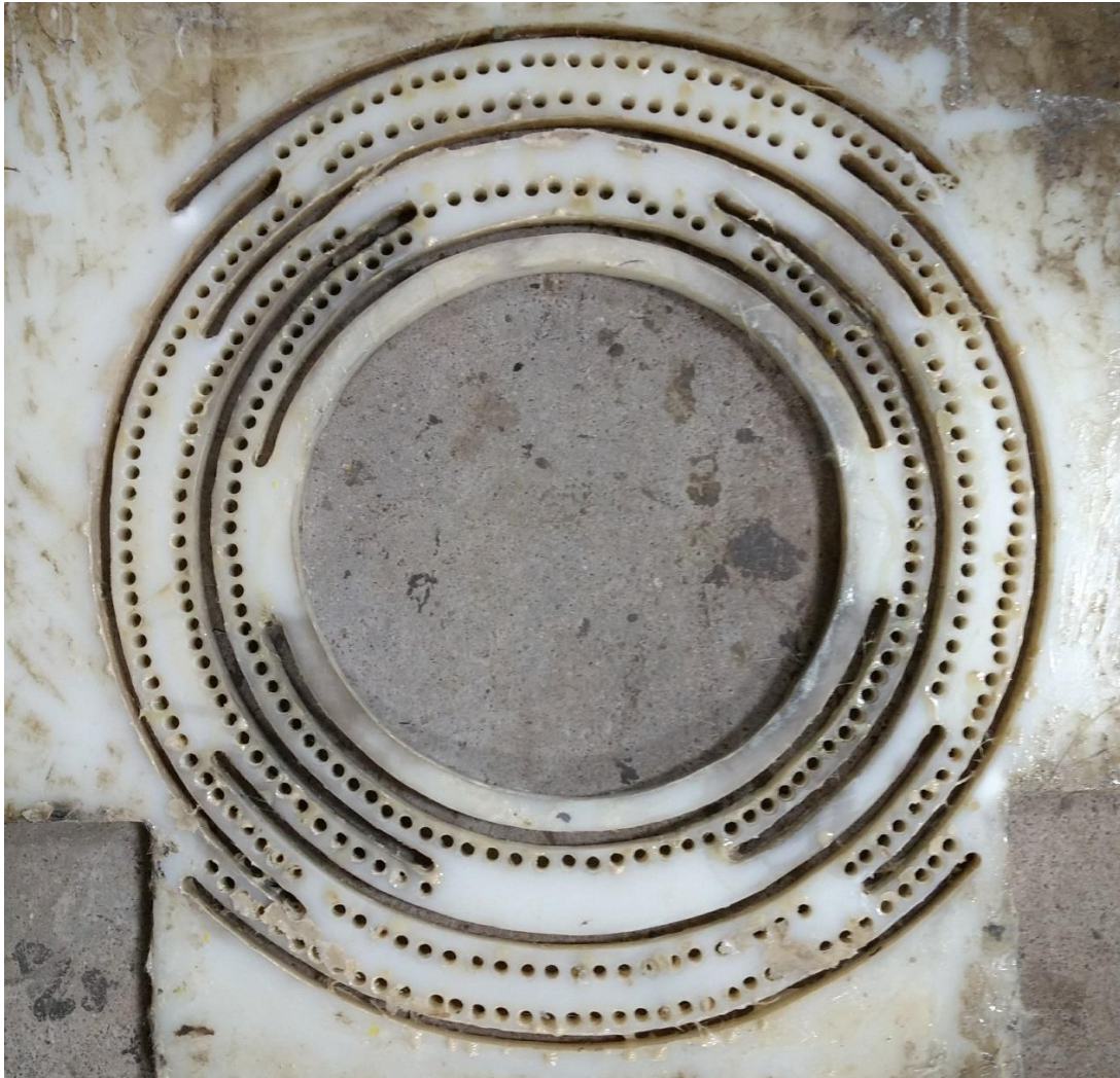
Figure 47 Preformer used for manufacturing GFRP pole
