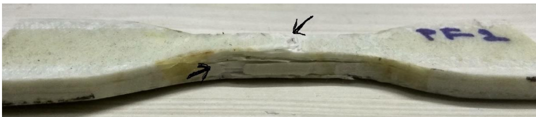
Figure 103 Shear plane rupture and delamination for pipe section specimens (type four)
