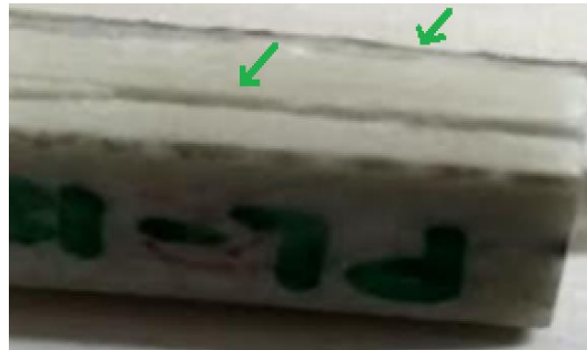
Figure 115 Delamination in compression strength test of pipe section specimens
