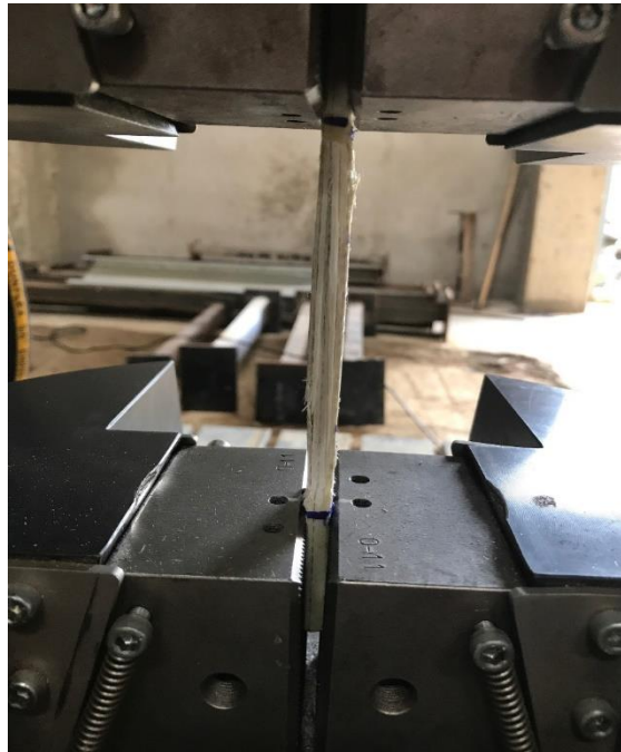
Figure 19 Fixture used for tension coupon testing
