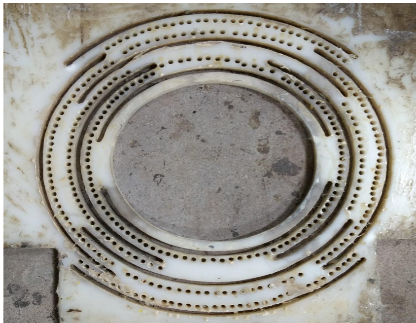
Figure 8 Preformer used for making pipe specimens
