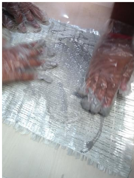
Figure 35 Application of resin in mats
