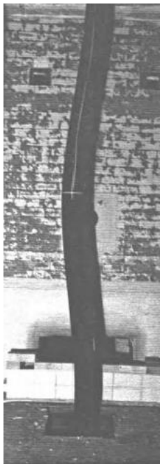
Figure 10- Deformed shape after exposure to standard fire, for column C-05
