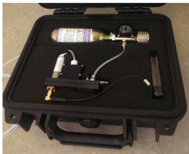
Figure 2.4: Photograph of a MEMS GC system components [4]
