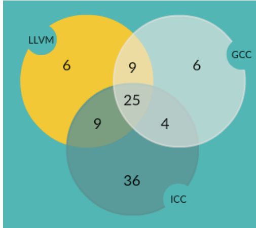
Figure 2.5: Comparison of number of vectorized loop kernels of TORCH and MiBench.
