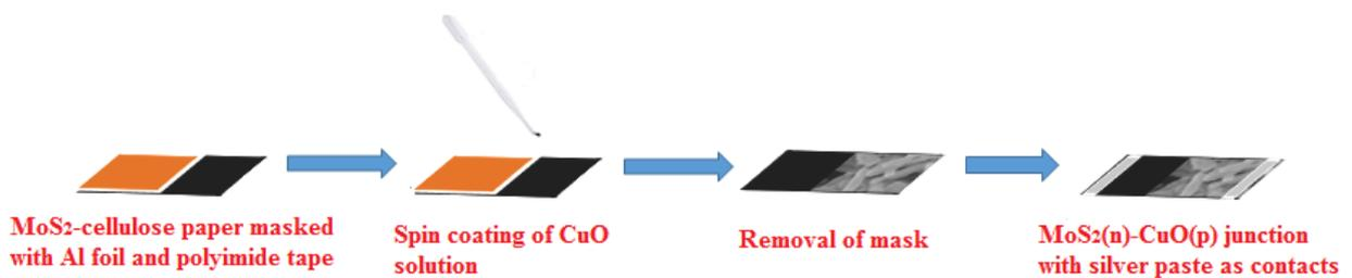
Figure 6.1: Schematic of the synthesis of MoS<sub>2</sub> on cellulose paper, hollow CuO nanorods and fabrication of MoS<sub>2</sub>-CuO piezotronic diode
