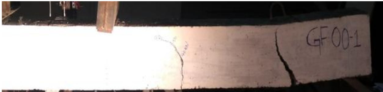
(b) GFRP Reinforced Beam
