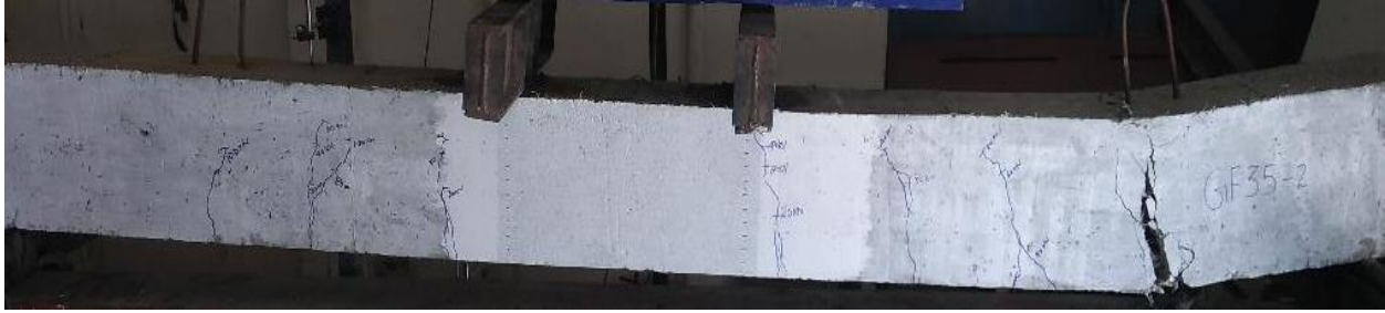
(c) GFRP Reinforced Beam with 0.35% PO Fiber
