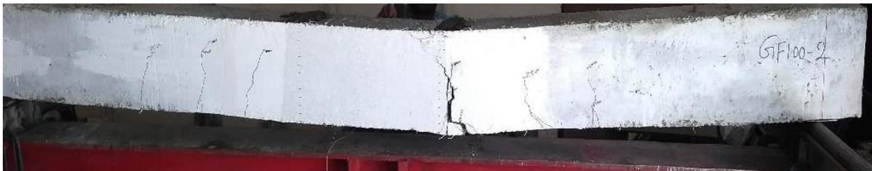
(e) GFRP Reinforced Beam with 1.0% PO Fiber
