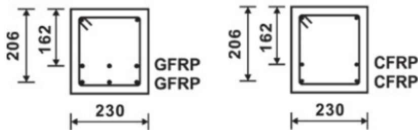
(b) Section details of beam with GFRP bars (left) and CFRP bars (right)
