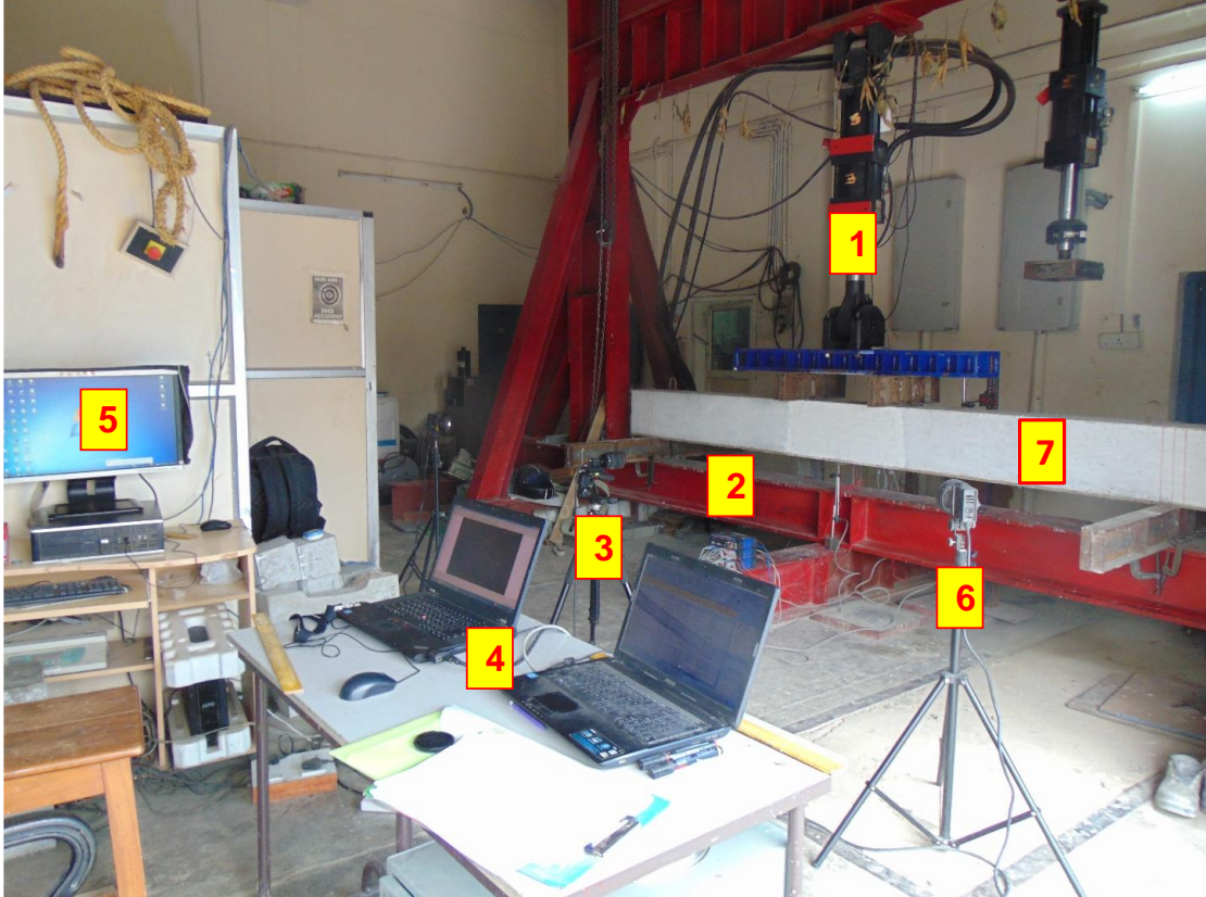
1. 250 kN MTS Actuator; 2.HBM DAQ system; 3. DIC camera; 4. DAQ Controller; 5. MTS Controls system; 6. Light source for DIC; 7. Test Specimen
