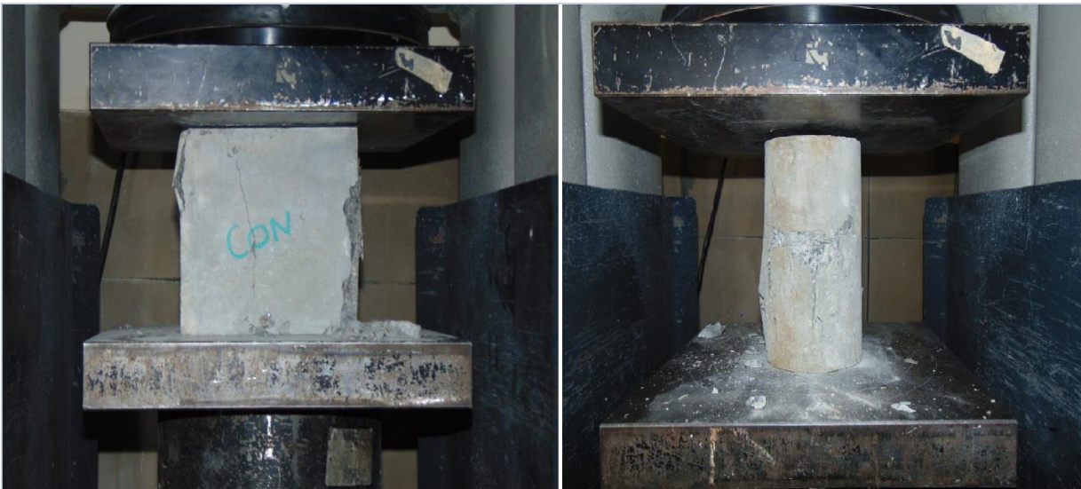
Figure 3. 2: Tested cube and cylinder
