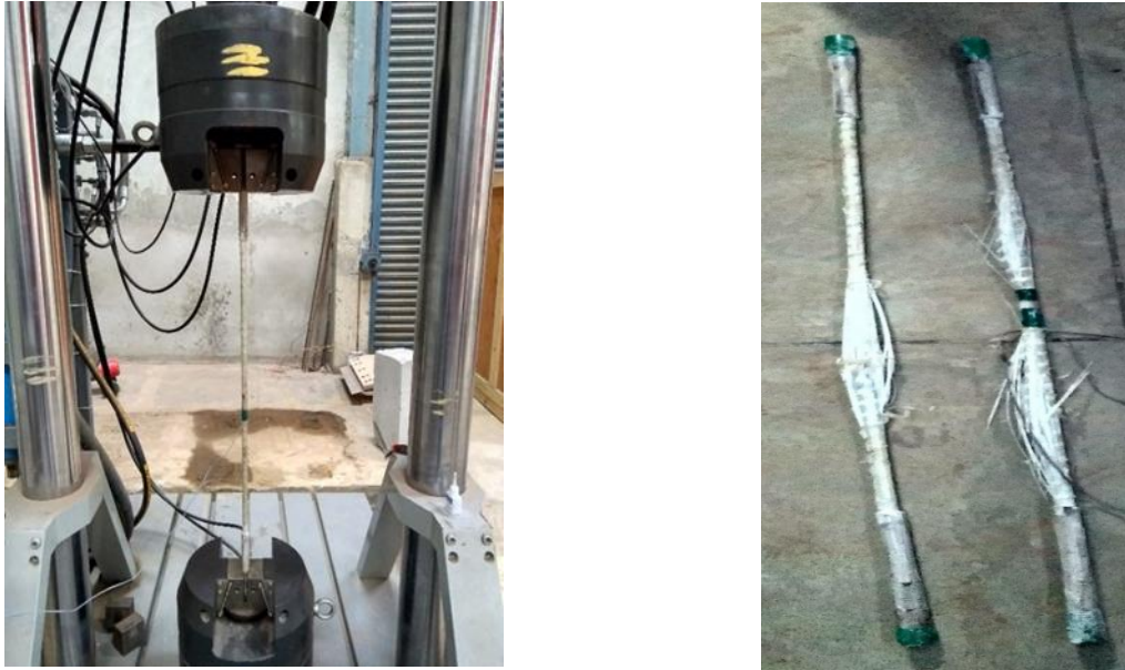
Figure 3. 5: Test setup for tensile test (left) and GFRP bars after failure (right)
