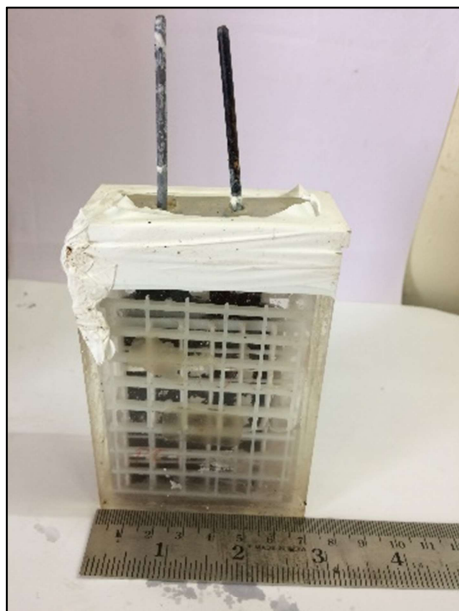
Figure 15: A laboratory prepared lead acid cell with negative limited.
