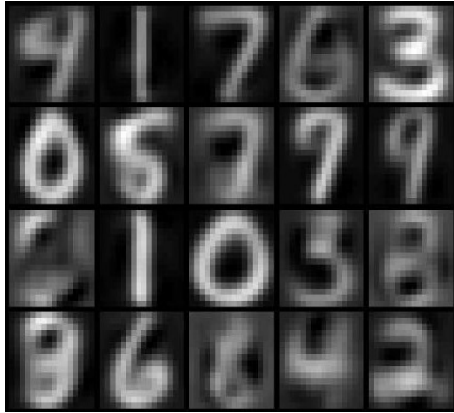
Fig. 3.1: The dictionary atoms obtained after learning USPS digit dataset
