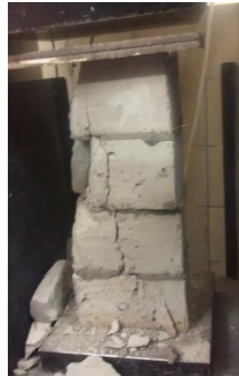
(c) Specimen after Compression Failure
