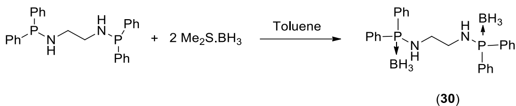
Scheme 4.3. Synthesis of the bis(amidodiphenylphosphine-borane) ligand 30
