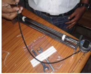
Figure 7 : Autogenous Shrinkage Test
