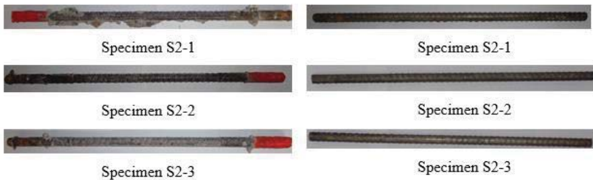
Figure 6: Rebars taken out from autopsied specimens of S2 series
