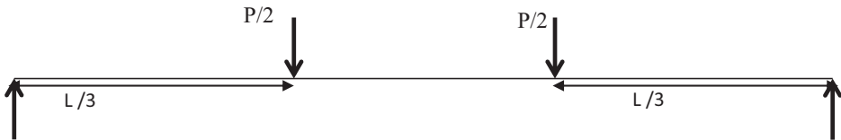
Fig. 6. Two point loading detail
