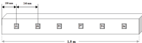
(a) Placement of PZT patch
