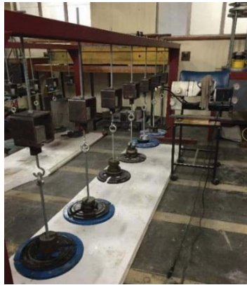
Figure 4: Time-dependent pull-out creep test setup
