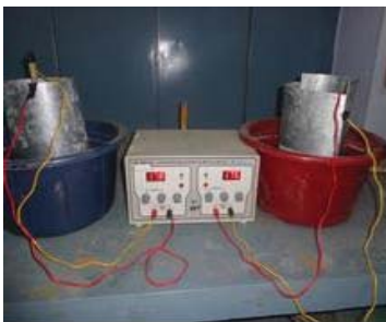
(a) Corrosion cell connected to meter
