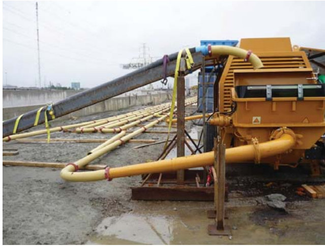
Figure 1: Layout of the closed-loop pumping circuit with a total length of 600 m
