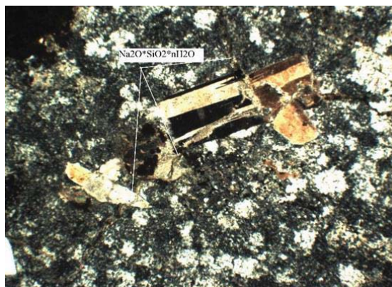
Figure 2: Propagation of alkali-silica hydrogel along the crack in the aggregate and the matrix (photo in the polarized light)
