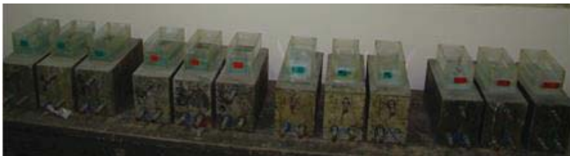
Figure 2: ASTM G 109 test specimens under continuous wetting and drying cycles
