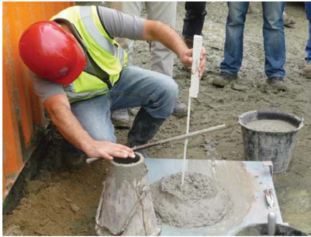
Figure 2: Slump measurement on fresh concrete at construction site
