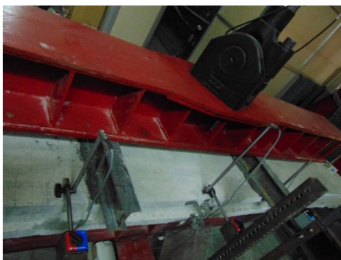
(a) Placing of LVDT's
