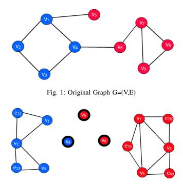
Fig. 2: HMRF model of G indicating anomalous node  $v_4$ ,  $v_5$  and  $v_6$
