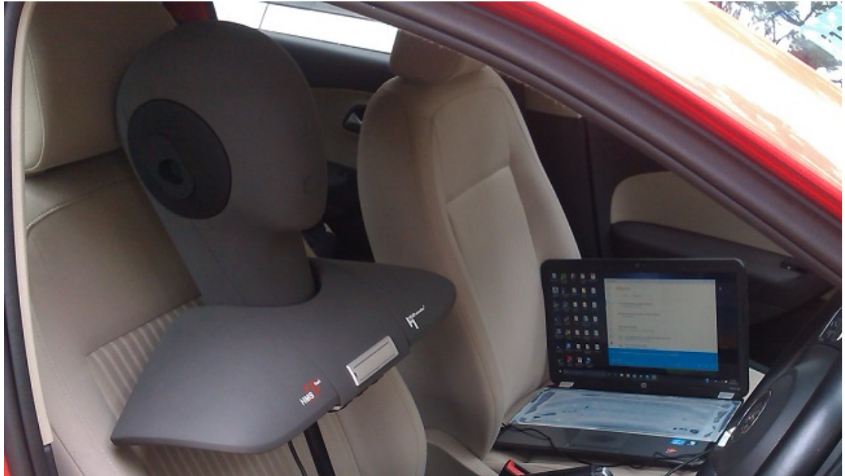
Figure 4.2: A test setup for recording the sound samples using HMS
