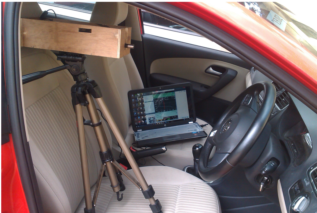
Figure 4.1: A test setup for measuring sound pressure levels using single microphone
