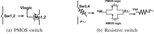
Fig. 5. Switch implementation using MOS
