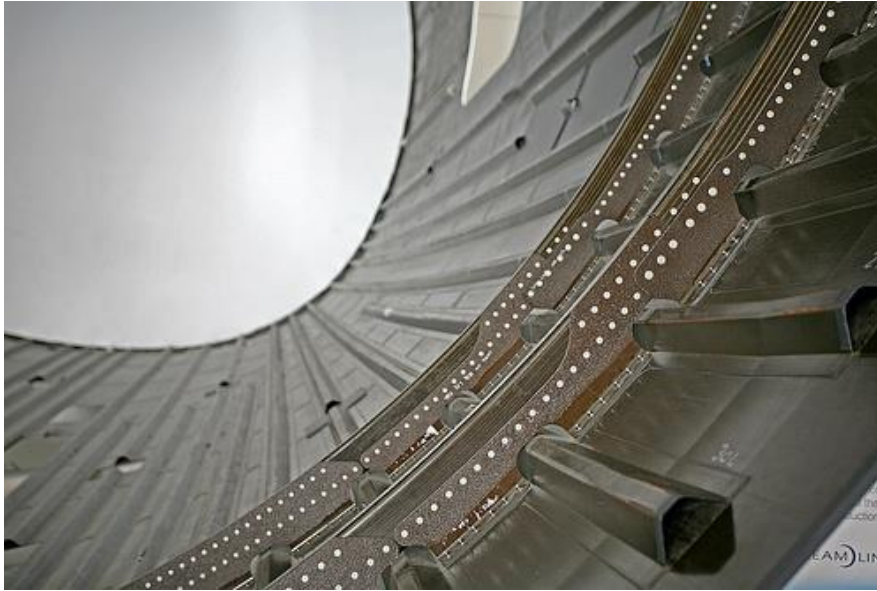
Figure 1.2: Disassembled fuselage section of Boeing 787 Dreamliner [3]
