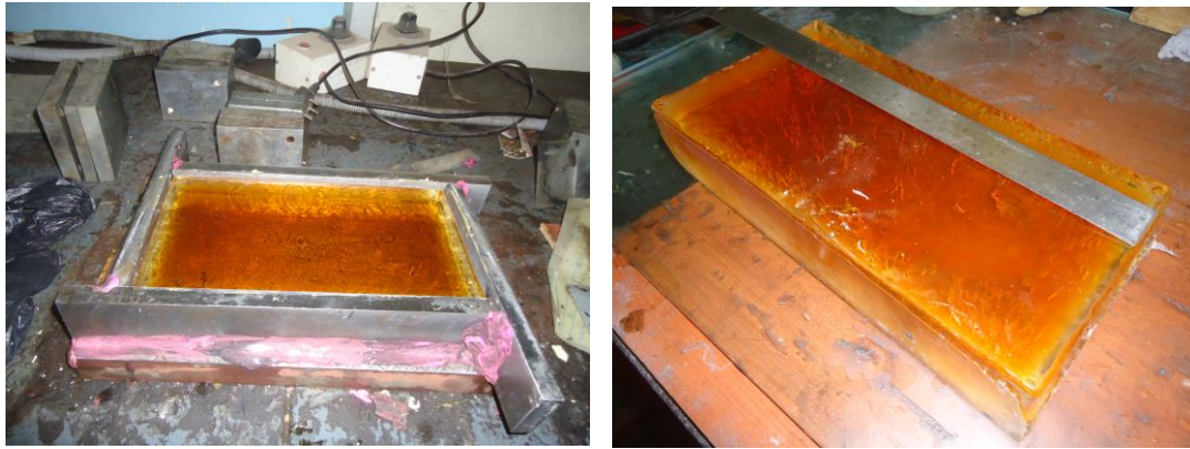
(a) (b) Figure 2.15: Casting of epoxy resin block using metal mold: (a) resin in mold while curing, (b) Cured resin block
