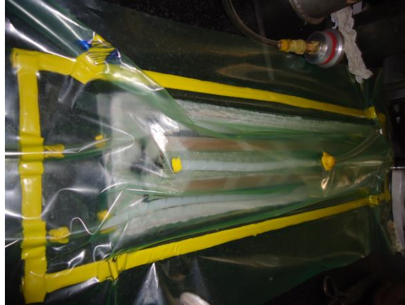
Figure 2.7: Sealing to the entire VI setup in vacuum cover
