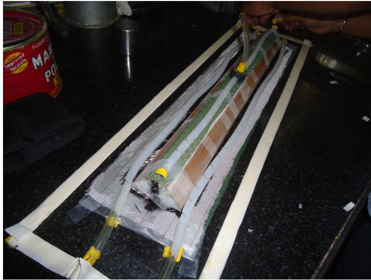
Figure 2.5: Setup of VI procedure: (a), (b) different stages of VI setup
