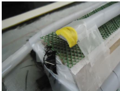
Figure 2.6: Closing of spiral free ends: (a) upper spiral tube (b) lower spiral tubes
