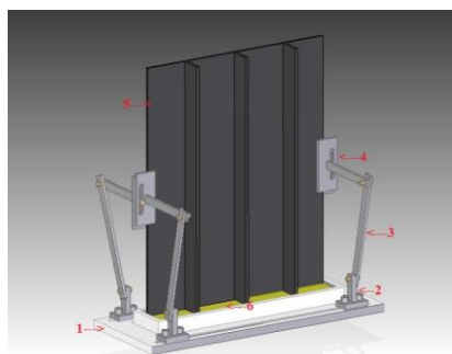
1. Base plate 2.Stand to hold links 3.Rotating link 4.Rotating arm 5.Stiffened panel 6.Resin pool
