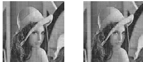
Fig. 3: For the original image of size 256 \times 256 in Figure 2, the image on the left is reconstructed via the new matrix and the right image is obtained via the corresponding Gaussian matrix with a down-sampling factor of four. This figure states that the constructed matrix provides competitive reconstruction performance.
