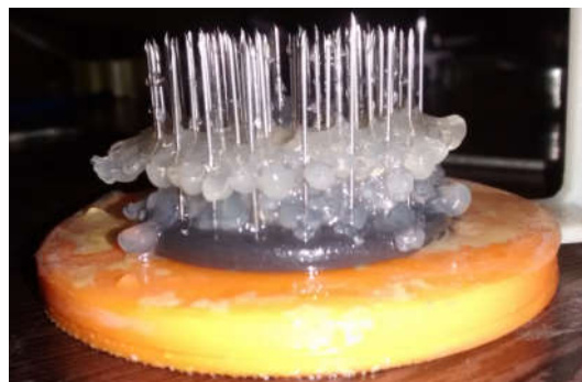
Figure 5.8 Successful multi-layer deposition with the help of vertical needles arrangement
