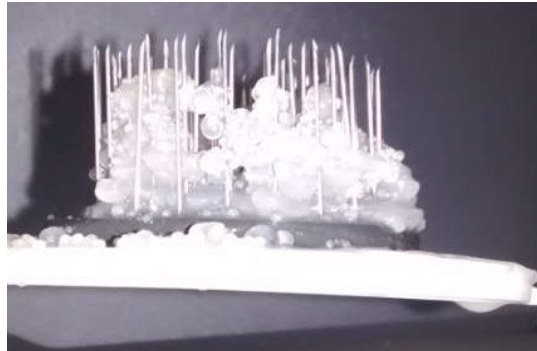
Figure 5.7 Vertical needle arrangement failed with high feed rates.
