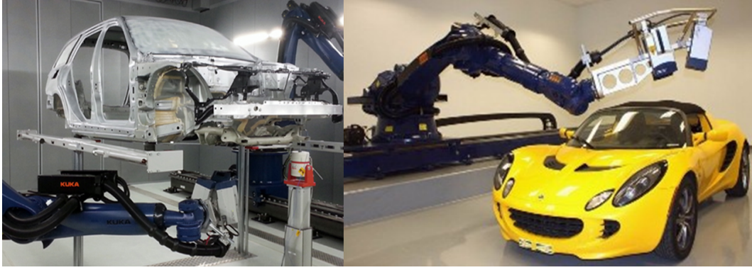
Figure 3.1: Laser Doppler vibrometer is used perform the modal analysis on the car bodies
