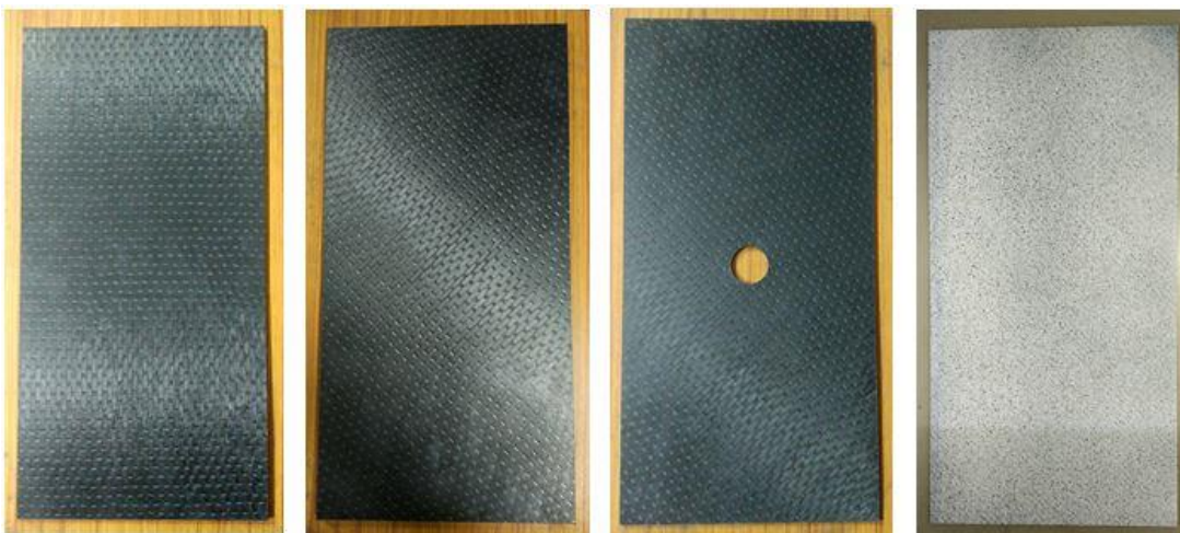
Fig 3.3: Stages of panel Fabrication using hand lay-up followed by vacuum bagging technique (a) CFRP plies are stacked using matrix (b) breather sheet is placed over the CFRP plies (c) Aluminium plate is placed on top of breather (d) everything is covered with plastic cover and vacuum is applied.
