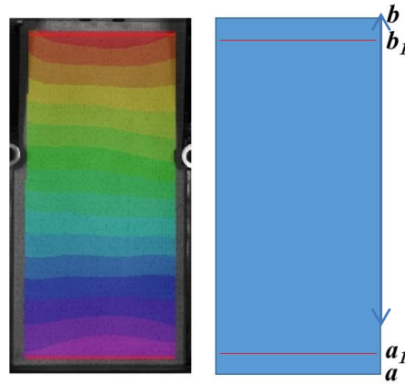
Fig 3.10: Axial displacement contour with axial displacement extracting lines.
