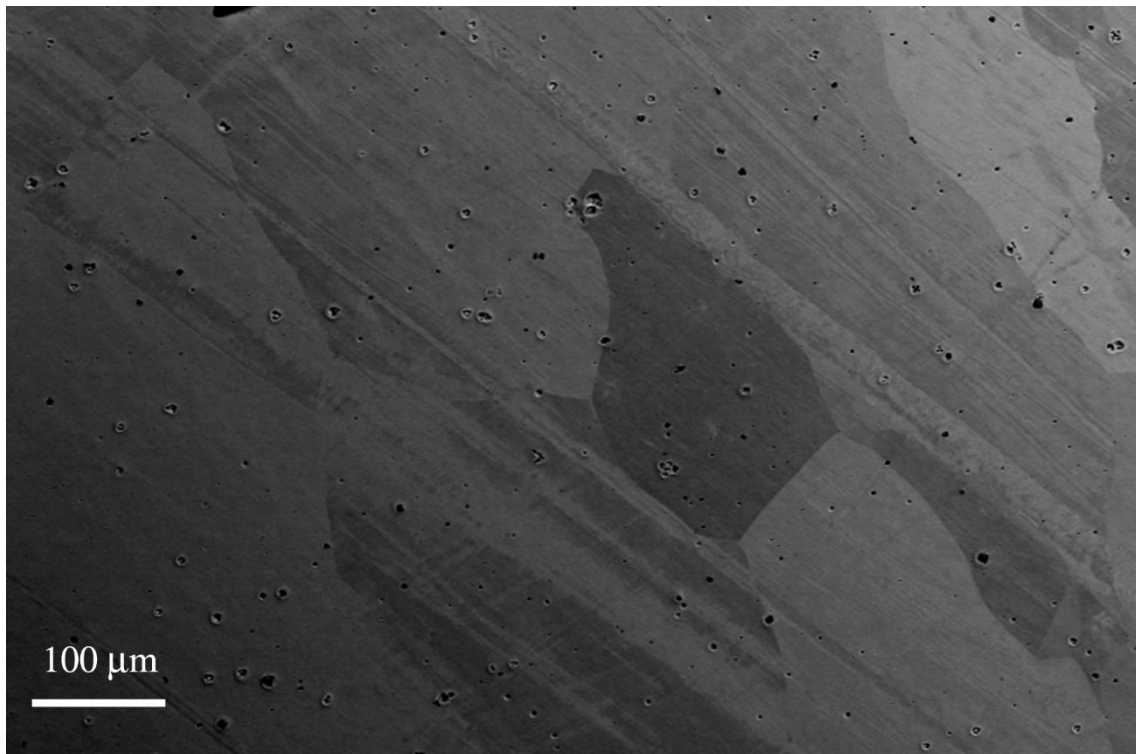
Fig.4.2: BSE micrograph of the homogenized CoCrFeMnNi HEA.
