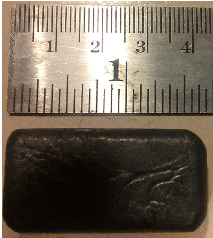
Fig. 3.1: As-received homogenized slab of the CoCrFeMnNi HEA used in the present research.
