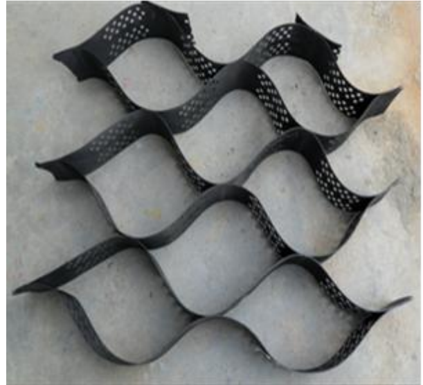
Figure 2. Typical geocell used in the study
