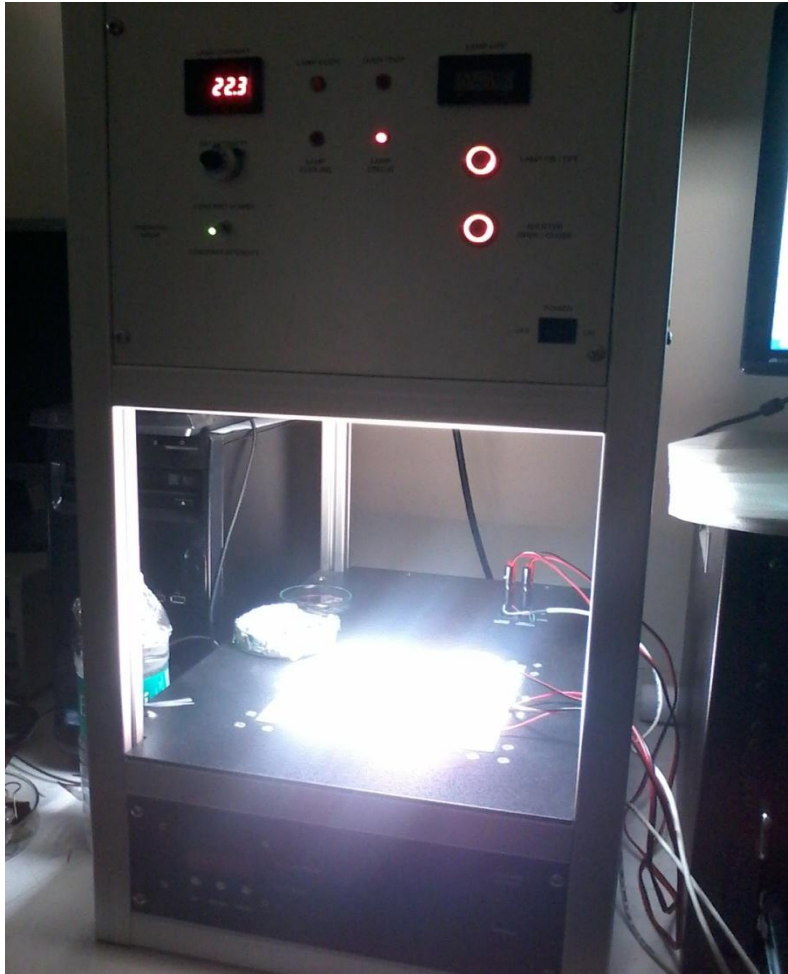
Figure 36 Testing in progress in a solar tester
