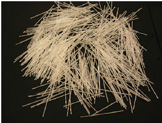
Fig. 1 Structural polypropylene fibers.
