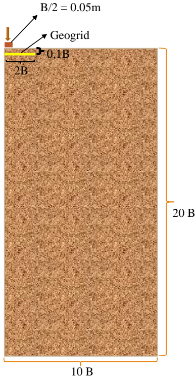
Figure 4.8: Schematic of the model on homogeneous medium with single layer of reinforcement
