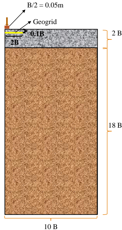
Figure 4.15: (a) Schematic model of two layers soil system with single layer of reinforcement condition
