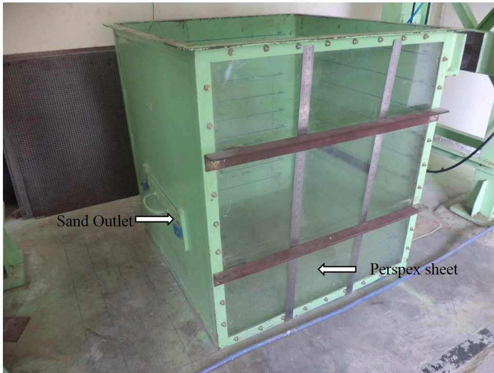
Figure 3.2: Soil chamber (900*900*1000) mm
