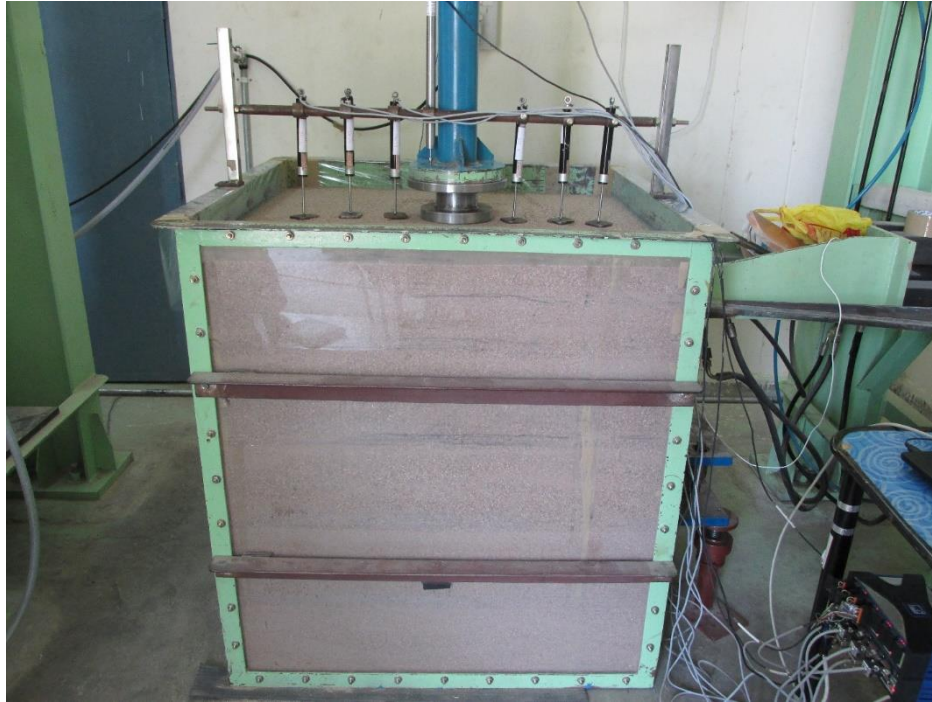
Figure 3.9: Determining the Modulus of elasticity of sand bed experimentally
