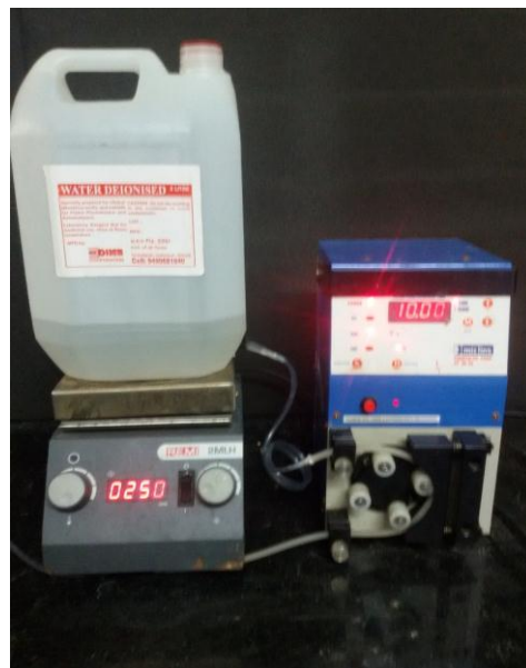
Fig 3.4.4 Peristaltic pumping system
