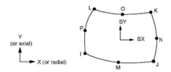
Fig. 4 Geometry of PLANE 183 finite element
