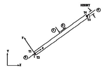
Fig. 3 Geometry of BEAM3 finite element
