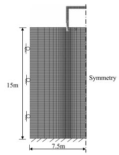
Fig. 6 Finite element meshing for Case 2 and Case 3
