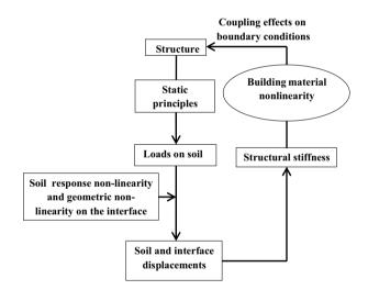
**Fig.1** Flow chart for soil-structure interaction [2]
