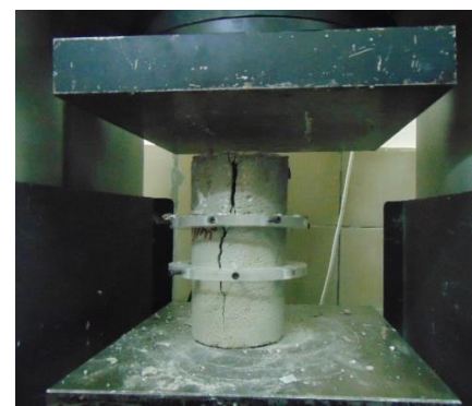
(d) Failed Specimen under Compression
