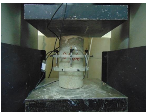
(c) Testing set-up with LVDTs
