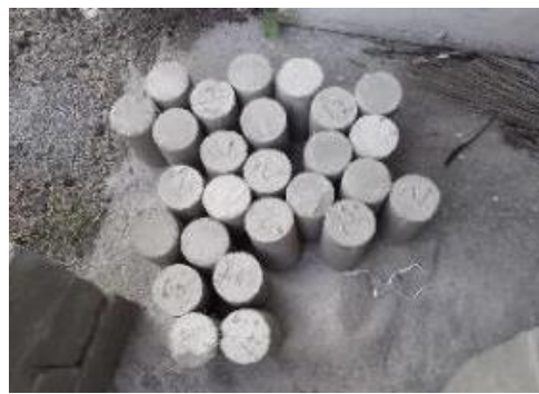
(e) Curing of cylinders
