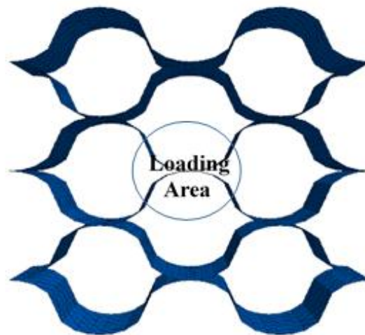
Figure 4.2: Honeycomb shaped geocell model in FLAC 3D
