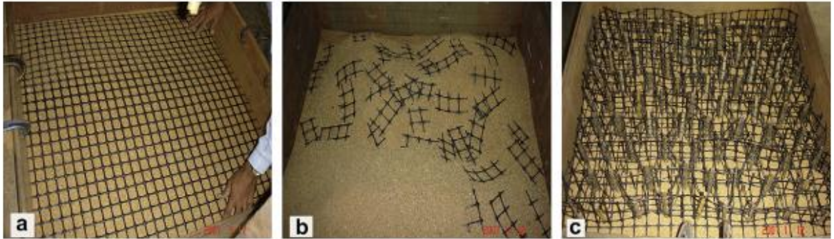
Fig. 4. Geosynthetics in different forms used for reinforcement: (a) planar layers, (b) randomly distributed mesh elements and (c) geocell layer.
