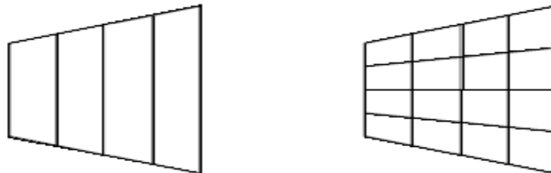
Figure 2.5: 1d (left) and 2d (right) Finite Volume discretization of an expanding domain
