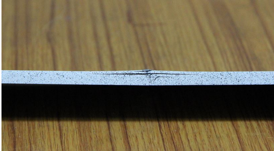
Figure 1.3: Multiple delaminations in CFRP
