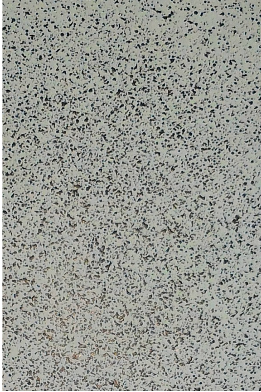
Figure 3.2: Zoomed view of specimen showing the speckle pattern
