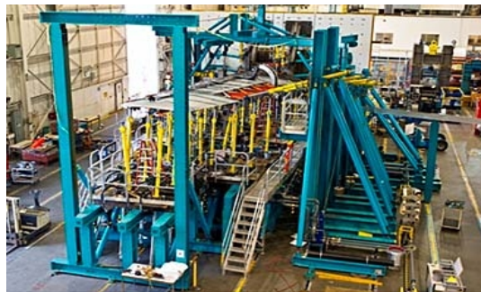
Figure 2.1: Full-Scale Fatigue Testing of the F/A-18 Fighter Aircraft [5]
