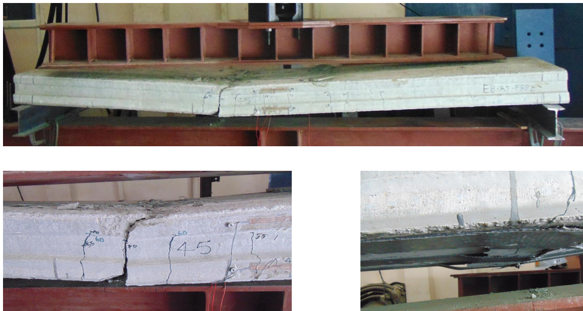
Figure 4.3: Mode of failure - I-S-150-7.5-EB-0.36-0.947
