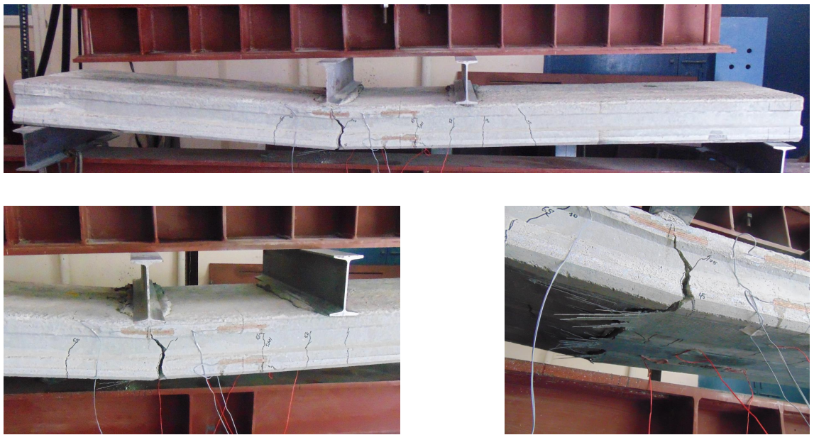
Figure 4.2: Mode of failure - I-S-150-7.5-EB-0.36-0.548
