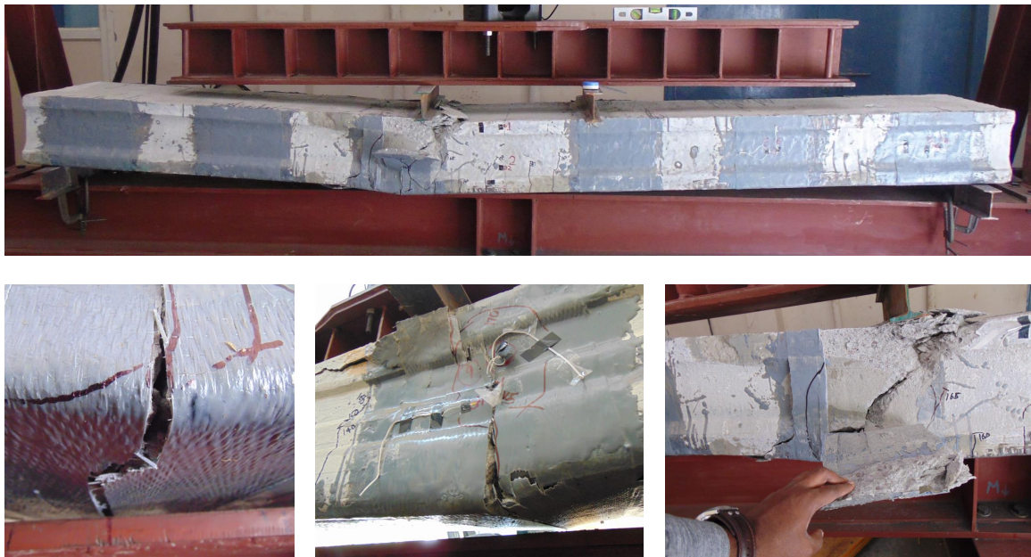
Figure 4.11: Mode of failure - II-S-250-5.4-EB-0.372-0.549
