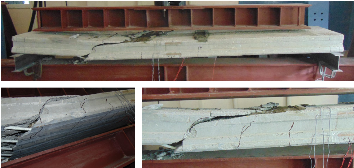
Figure 4.5: Mode of failure - I-S-150-7.5-NSM-0.36-0.94
