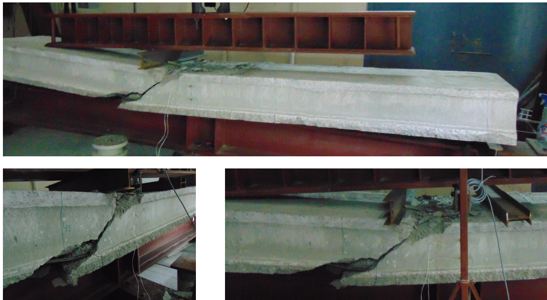
Figure 4.10: Mode of failure - II-C-250-5.4-0-0-0 (control)
