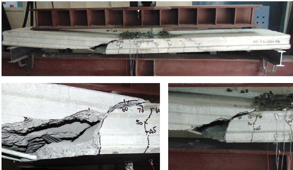
Figure 4.4: Mode of failure - I-S-150-7.5-NSM-0.36-0.564
