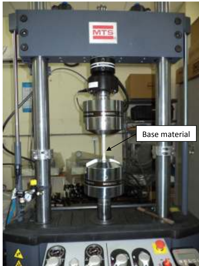
Fig. 8 Tensile testing of the Base material
