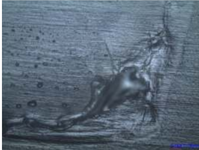
Fig. 12 Stagnant solid material near the bottom of the seam at the retreating side of the joint at 1000rpm and tool pin temperature of 40°C
