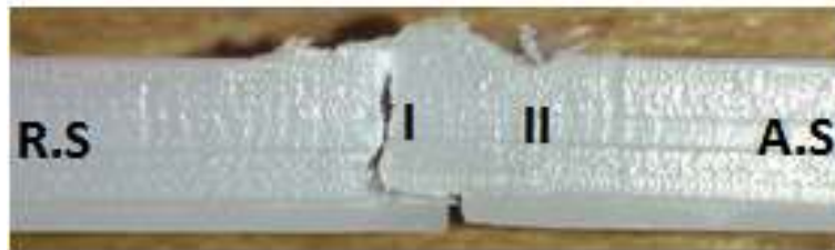
Fig. 23 Representation of deformation zones in the transverse section of a tensile-tested sample.
