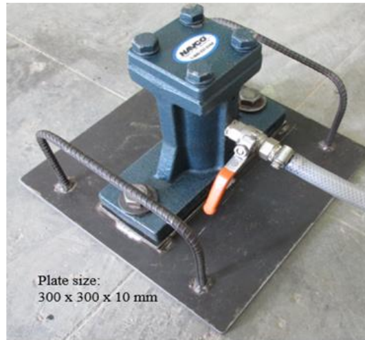
Fig 4.2: Pneumatic vibrator used for compaction
