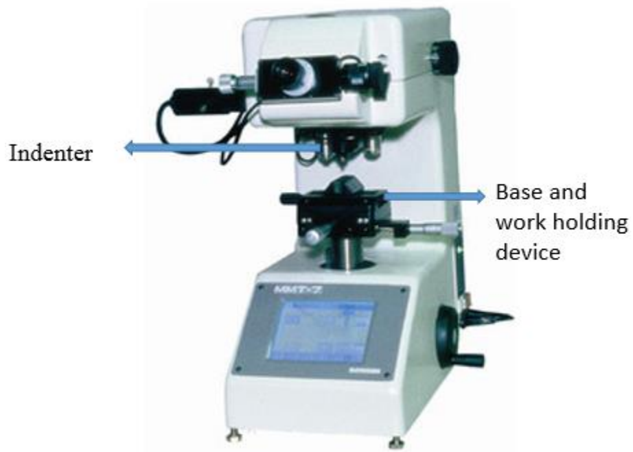
Figure 8(b) –Hardness testing setup.
