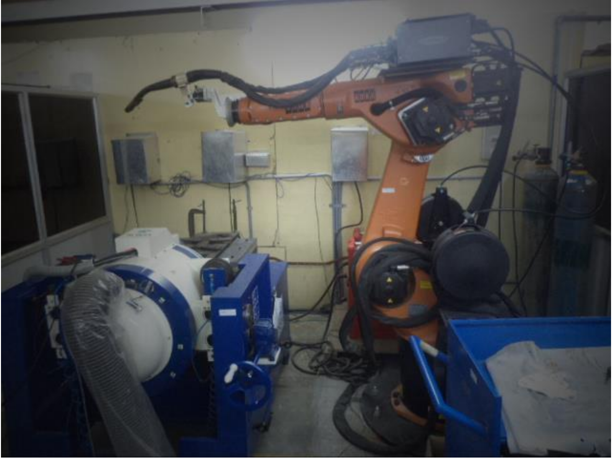
Figure 8(a)-Experimental set-up of twin wire welding.
