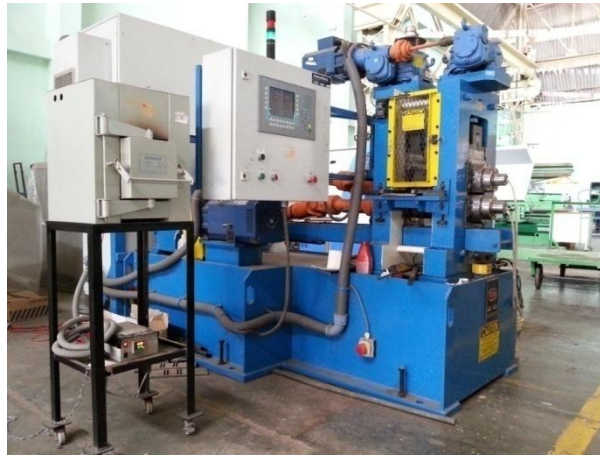
Fig. 2: Rolling machine and muffle furnace setup
