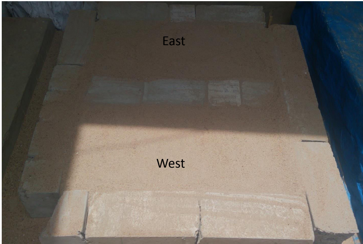
Fig.3.31: Test-pit after completely filling with sand
