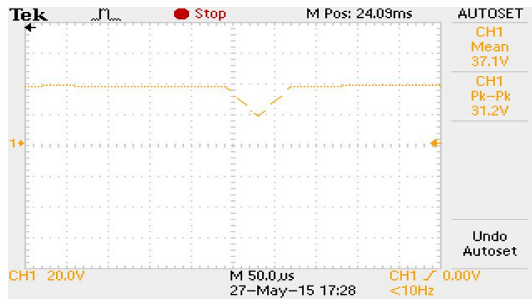
Figure 4.12: Output voltage under load transient
