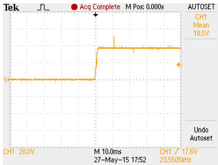
Figure 4.10: Output voltage under line transient
