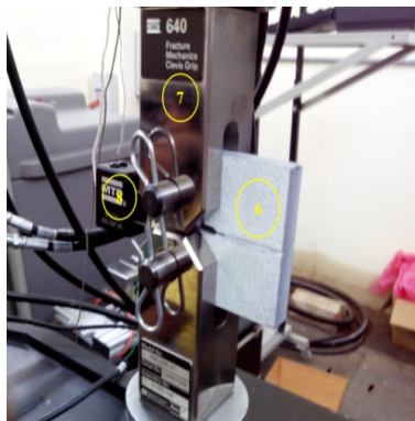
Figure 5.6: Loaded CT specimen
