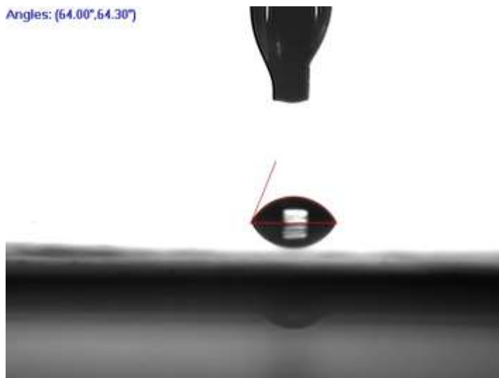
Figure 6.17: SU-8 2002 + Glycidol film after Cu etchant treatment
