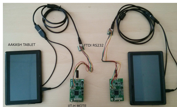
Figure 1.2: Text messaging between two android devices (Aakash tablet) through IIT-H motes
