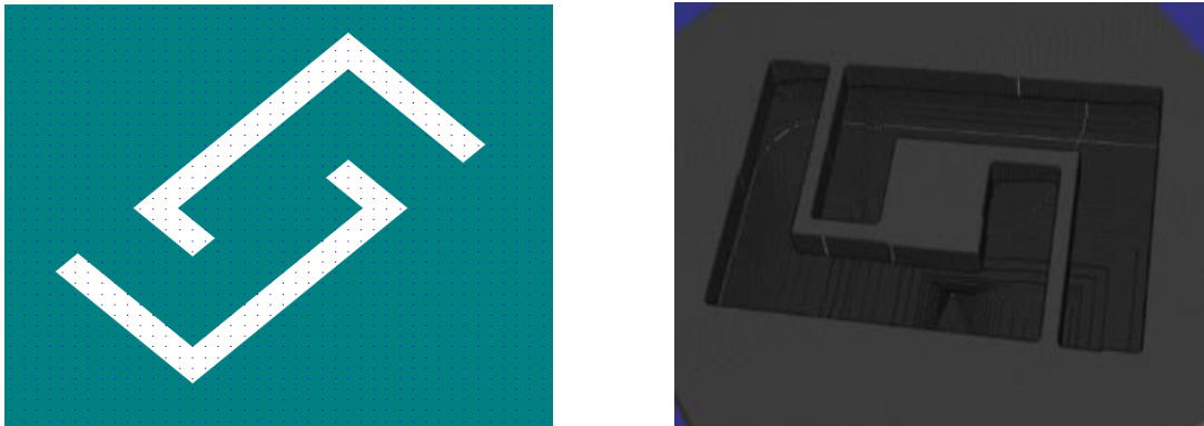
Fig.5.8: showing the mask used and the bolometer sensor membrane obtained using Intellisuite based FABSsim physical simulation
