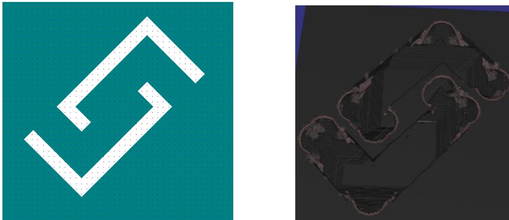
Fig.5.3: showing the mask used and the bolometer sensor membrane obtained using Intellisuite based FABSIm physical simulation.
