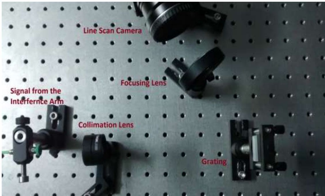
Figure 3.6: The spectrometer set-up in lab
