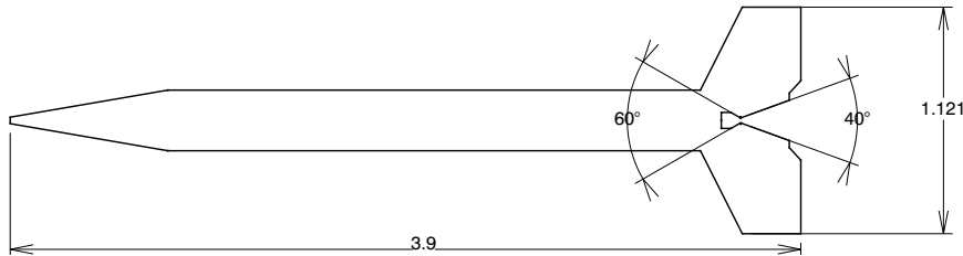
Figure 4.1: Schematic of Sonda II rocket [1] (dimensions in meters)
