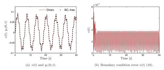
Figure 3. Comparison of direct numerical solution z(t) and solution obtained using the Galerkin method  $y_1(0,t)$  for (34). The parameters are  $b_1 = 0.01$ ,  $b_2 = b_3 = \alpha = 1$ ,  $b_4 = 0$ ,  $\beta = F = 0.5$ ,  $\omega = 2\pi$ , and N = 7.
