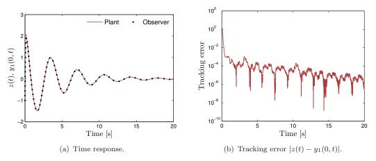
Figure 7. Comparison of plant output z(t) and observer output  $y_1(0, t)$  for (38). N = 20 terms were used in the Galerkin approximation.
