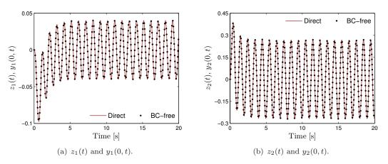
Figure 1. Comparison of direct numerical solution  $z_i(t)$  and solution obtained using the Galerkin method  $y_i(0,t)$  for (31). The parameters are  $b_1 = b_6 = 2$ ,  $b_2 = b_4 = \alpha_{22} = 1$ ,  $b_3 = b_7 = b_8 = \alpha_{11} = 0.1$ ,  $b_5 = 0.75$ ,  $\alpha_{12} = 0.3$ ,  $\alpha_{21} = 0.5$ , F = 1.8,  $\omega = 2\pi$ , and N = 7.
