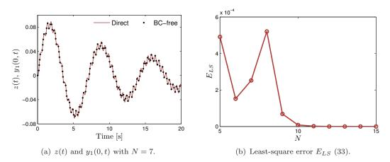
Figure 5. Comparison of direct numerical solution z(t) and solution obtained using the Galerkin method  $y_1(0,t)$  for (34) when the velocity delay term is nonzero. The parameters are  $b_1 = 0.05$ ,  $b_2 = 0.75$ ,  $b_3 = \alpha = F = 1$ ,  $b_4 = 0.1$ ,  $\beta = 0.5$ , and  $\omega = 4\pi$ .
