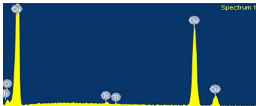
Figure 7. EDS of Cu-10 g l -1 TiO 2 deposited sample at 5 A dm -2 .
