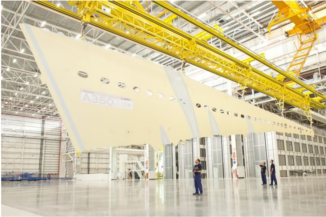
Figure 1.2: Wing covers of Airbus A350 XWB made of CFRP [1]
